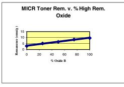
Figure 6. Variation of remanence to % oxide B
